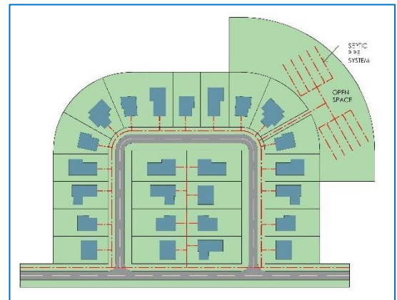
Figure 13 - Localized Sewer Distribution allows higher density on a short-term and extension of sewer system in the long term.
